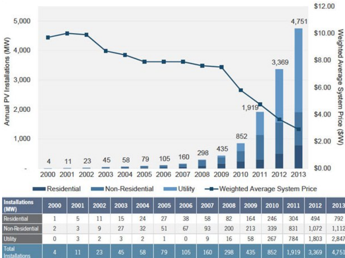
Figure 3. - U.S. PV Installation and Average System Price, 2000-2013 (Solar Energy Industries Association/GTM Research, 2014)
